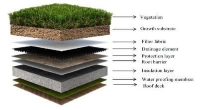
Typical components of a green roof.
